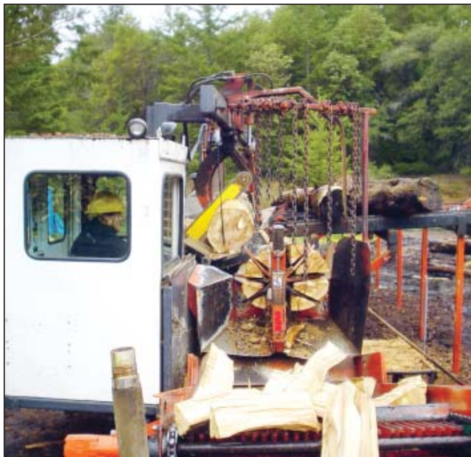
Frank Vaine Logging & Firewood uses this Multitek 3040XP90 firewood processor to produce cut, split firewood; machine uses an overhead grapple to move logs firmly and securely into position to be bucked.
