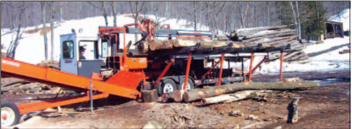
Gish Logging operates four Multitek 2040 firewood processing machines.
