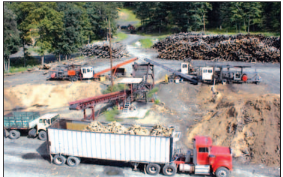
Overview showing three Multitek firewood processors feeding conveyors at Gish Logging's firewood operation.
